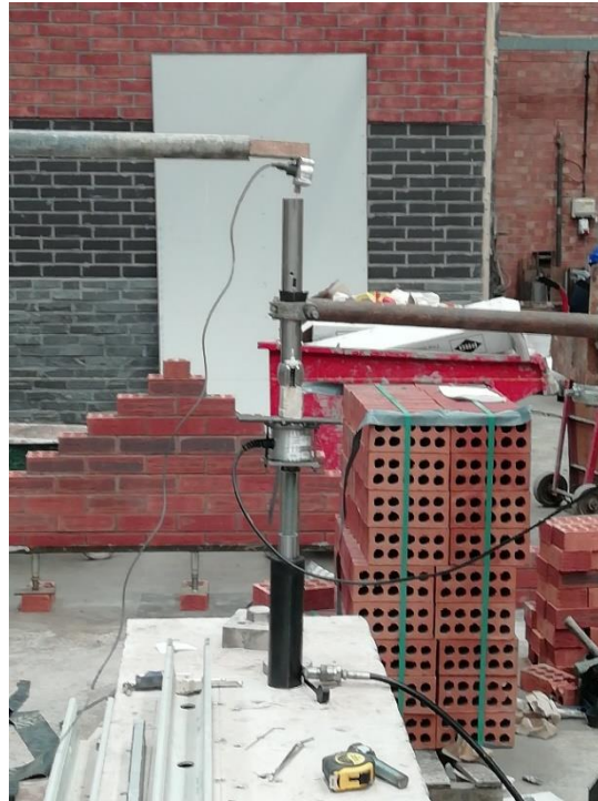
Plate 1 - Typical Test Set-Up Vertical Loading
