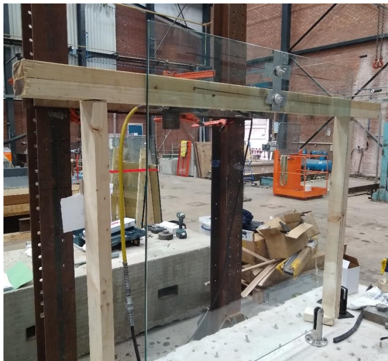
Plate 2 – Test 1 – 12 mm Toughened Glass – Deflection Measurement Side
