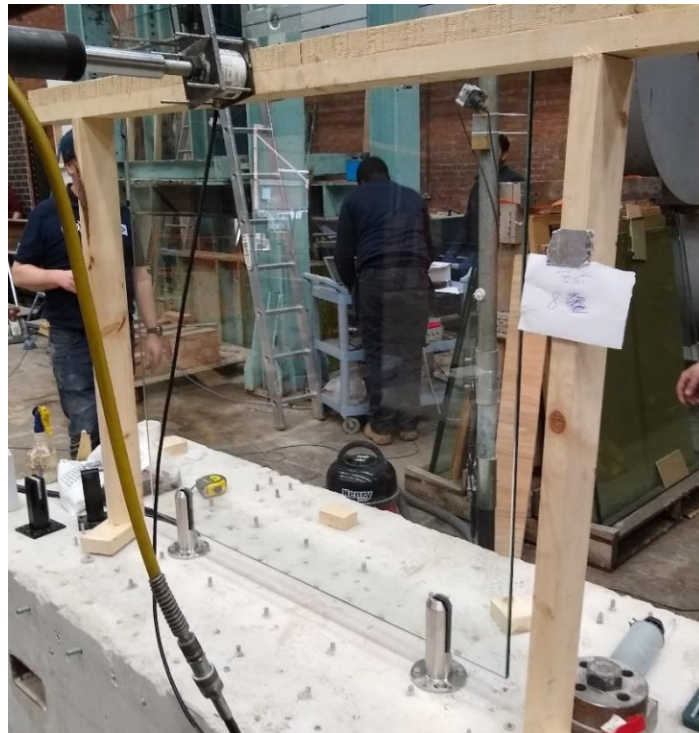
Plate 1 – Test 1 – 12 m Toughened Glass – Load Application Side
