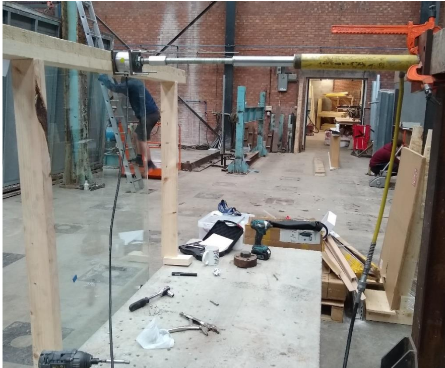
Plate 1 – Test 1 – 15 mm Toughened Glass – Load Application Side
