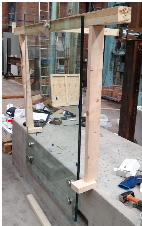
Plate 4 – Test 3a – 21.5 mm PVB Toughened Laminated Glass – UNI 10806 Test
