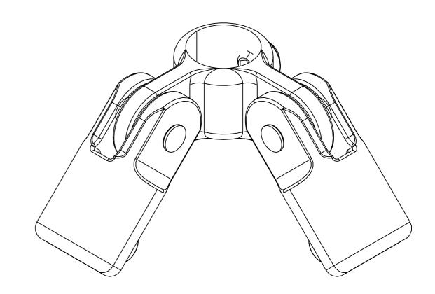
A double corner swivel connector typically used for sloping guradrail. This fitting combines 1 x 168M & 2 x 173F. The swivels can travel approximately 85° from the horizontal in both directions. THIS FITTING IS NOT DESIGNED TO WITHSTAND LATERAL LOADINGS. AN ENTIRE STRUCTURE SHOULD NOT BE BUILT USING ONLY SWIVEL FITTINGS, THIS WOULD BE UNSTABLE.
