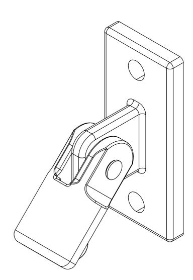
Non-structural male locating swivel. This fitting combines 1 x 169M & 1 x 173F. The swivel can travel approximately 85° from the horizontal in both directions. THIS FITTING IS NOT TO BE USED AS A BASE PLATE FOR GUARDRAIL. THIS FITTING IS NOT DESIGNED TO WITHSTAND LATERAL LOADINGS.
