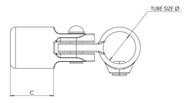
Single inline swivel connector. Typically used on sloping guardrail. This fitting combines 1 x 173M & 173F. The swivels can travel approximately 85° from the horizontal in both directions. THIS FITTING IS NOT DESIGNED TO WITHSTAND LATERAL LOADINGS. AN ENTIRE STRUCTURE SHOULD NOT BE BUILT ONLY USING SWIVEL FITTINGS, THIS WOULD BE UNSTABLE.
