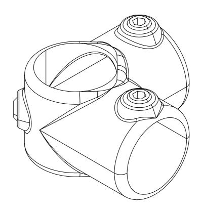
Typically used on straight and level guardrail to connect the mid rails to the upright at a 90° corner. Normally used in conjunction with the 128 fitting when building two rail guardrail.
