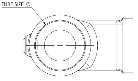
PART CODE MATERIAL TUBE SIZE ∅ С  $\emptyset$ **FINISH** В Ε Α D 16144B 33.7 96mm 45mm 65mm Malleable Cast Iron 104mm 67mm 14mm Galvanised 14mm 16144C 42.4 109mm 78mm 65mm 50mm Malleable Cast Iron 114mm Galvanised 16144D 48.3 120mm 123mm | 86mm | 65mm | 60mm 14mm Galvanised Malleable Cast Iron
