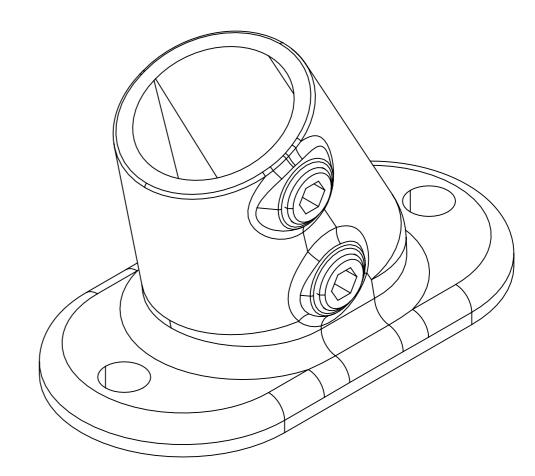
Similar to a type 152, it is used to set the upright at an angle between  $11^{\circ}$ – $30^{\circ}$ . This fitting should only be subjected to light loads which cannot be positioned at 90° to the applied load. For greater loads or other tube sizes a type 132 flange should be used with the upright bent to the required angle  $\varnothing$  indicates the diameter of the fixing hole.
