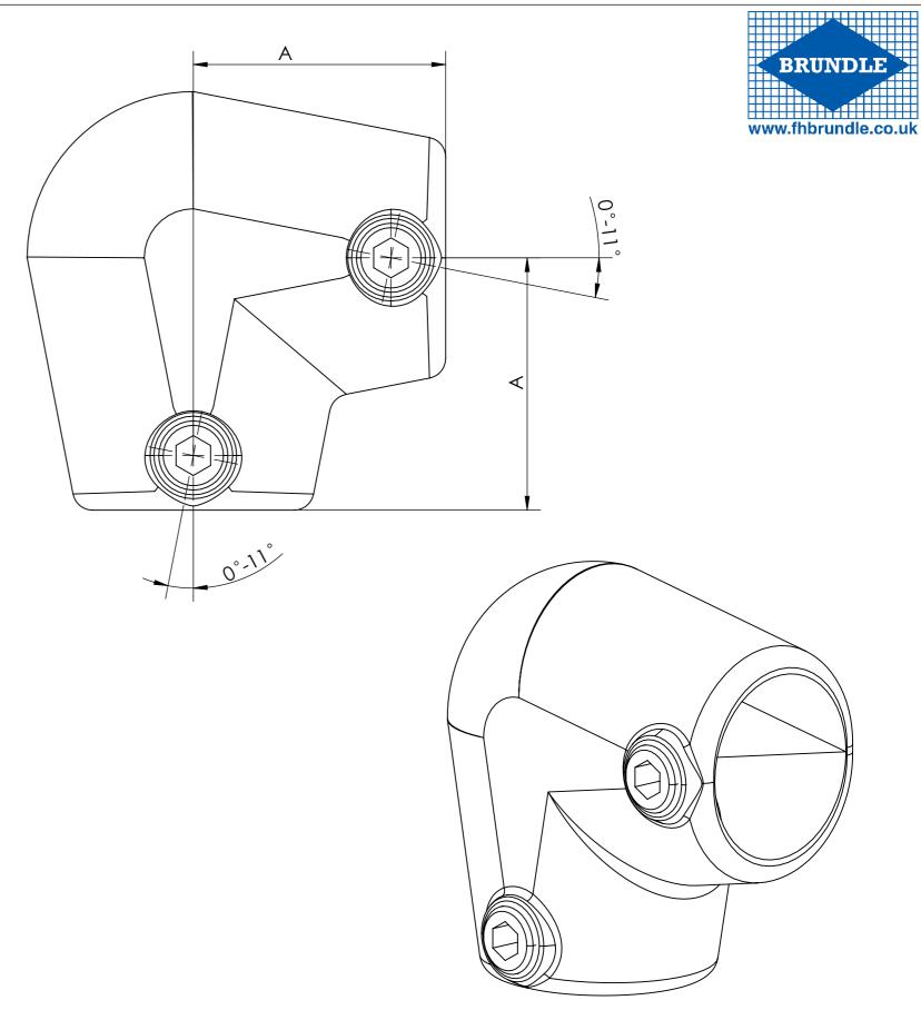
Typically used on shallow sloping guardrail between 0° and 11° at the start or end of a run to connect the upright to the top rail. This fitting can be used at either the bottom or top of an incline. Normally used in conjunction with the 153 fitting.
