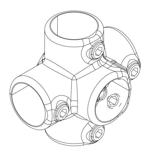
A Four Way Cross for joining tubes together in the centre of a structure. The fitting allows the upright to pass through the centre with the cross rails joining at 90° to the upright.
