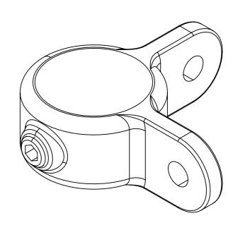
Double male fitting with the connection lugs at 90° to each other. This fitting can also be used to retain display panels etc. in place.
