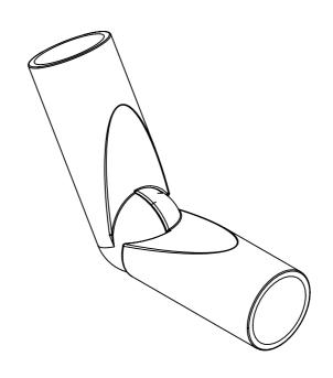
Fitting for creating an adjustable bend between the horizontal and the vertical.
