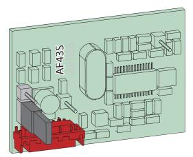
Radio-frequency control card for completing the receiving circuit fitted in all CAME control cards, while enabling it to receive radio signals coming from CAME transmitters.
