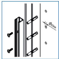
Anchor suitable for natural stone with dense dstructure.
