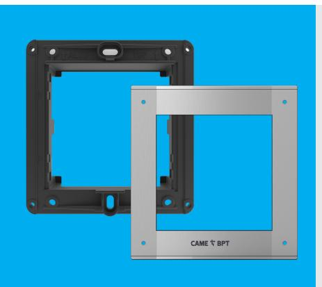
Frame and plaque for 1-module MTM. Black painted aluminum frame with cataphoresis finish ensures high resistance to corrosion and rust. Brushed anodised aluminium plaque.
