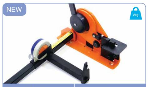
Code 43MC013X Practical Punch and Shear Tool W50 x D 175 x H 130 x 340mm Handle Length Max. Working Capacity Shearing – 20 x 3mm (flat strip), 5 (square bar), 5 (round bar/wire)
