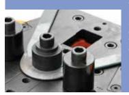
This simple but effective special bending pillar allows gradual and sharp angles in flat bar to be bent on edge. This is such a useful feature when making frames and components out of flat bar.
