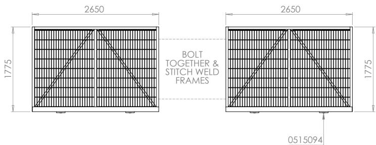
This 1.8m x 4M sliding track gate is delivered as two individual frames. The frames need to be welded and bolted together on site. The floor tracks then need cutting to a total length of 9365mm before fitting so it matches the total rolling distance of the gate. Goal posts, pales & gate fittings are provided so the gate can be fully assembled onsite.
