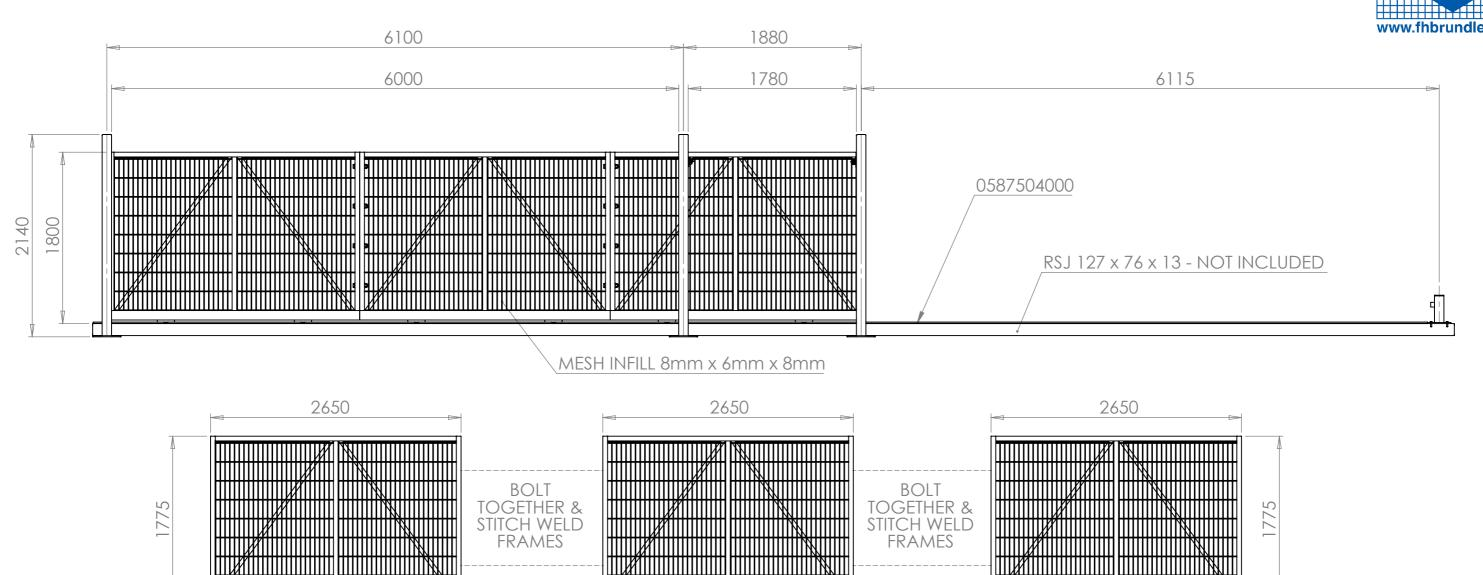
This 1.8m x 6M sliding track gate is delivered as three individual frames. The frames need to be welded and bolted together on site. The floor tracks then need cutting to a total length of 14115mm before fitting so it matches the total rolling distance of the gate. Goal posts, pales & gate fittings are provided so the gate can be fully assembled onsite.
