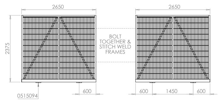
This 2.4m x 4M sliding track gate is delivered as two individual frames. The frames need to be welded and bolted together on site. The floor tracks then need cutting to a total length of 9365mm before fitting so it matches the total rolling distance of the gate. Goal posts & gate fittings are provided so the gate can be fully assembled onsite.
