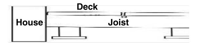
Allow proper spacing between deck boards for drainage, and expansion and contraction of the boards. A gap of 6mm each end for a 5.5m board is recommended to allow for linear expansion, pro rata for shorter boards. The hidden fastening system is already engineered for perfect spacing every time. Simply install grooved decking tight to the hidden fasteners.
