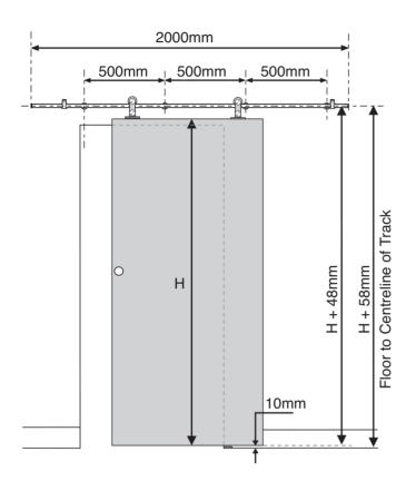
Notes: Must be installed into a solid wall
